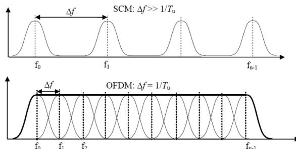
Fig. 2. Similarity and difference between an SCM (top) and an OFDM system (bottom)
