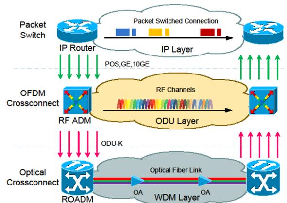
Fig. 4. Proposed DSON structure
