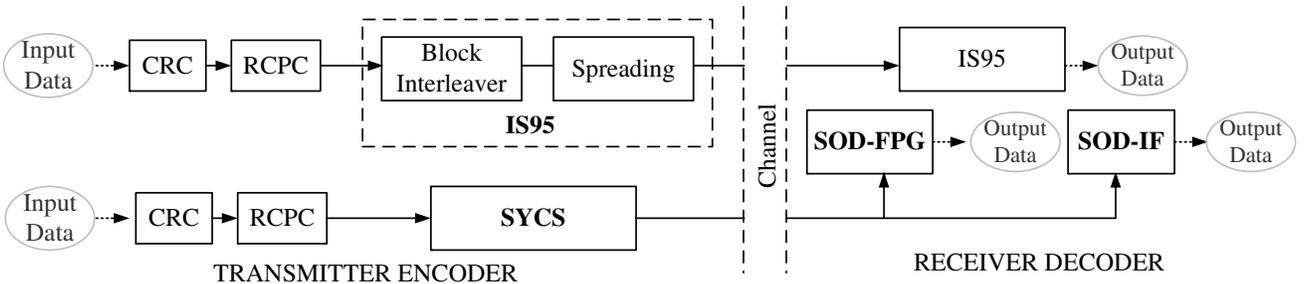
Fig. 7. Encoder and decoder block diagrams.
