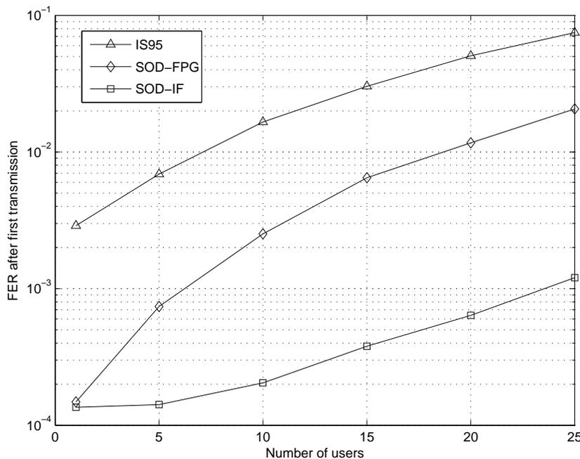
Fig. 8. Coded case with Rayleigh fading.
