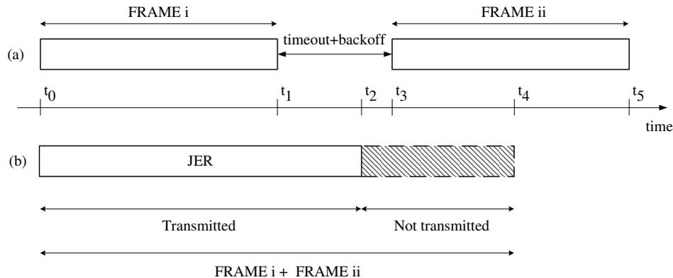
Fig. 2. (a) Hybrid Type II frame retransmission, (b) JER.
