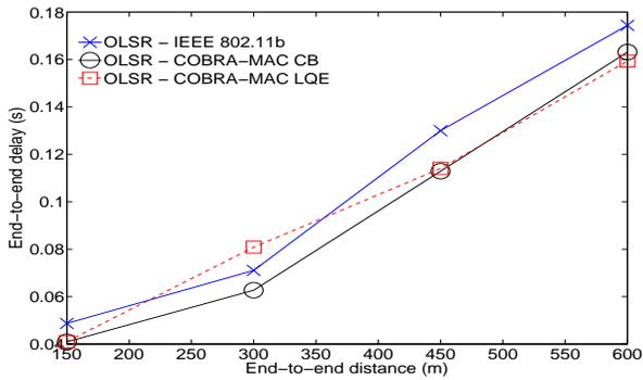
Fig. 63. End-to-end delay vs. End-to-end distance, linear topology, inter-node distance is 30 m, offered load is 2 kBps.
