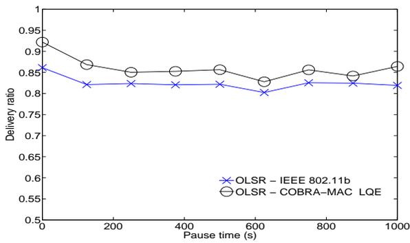
Fig. 98. Delivery ratio vs. Pause time, random waypoint mobility model, area is 320 m X 320 m, 20 nodes, 10 sources.
