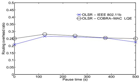
Fig. 103. Routing overhead ratio vs. Pause time, random waypoint mobility model, area is 320 m X 320 m, 30 nodes, 20 sources.
