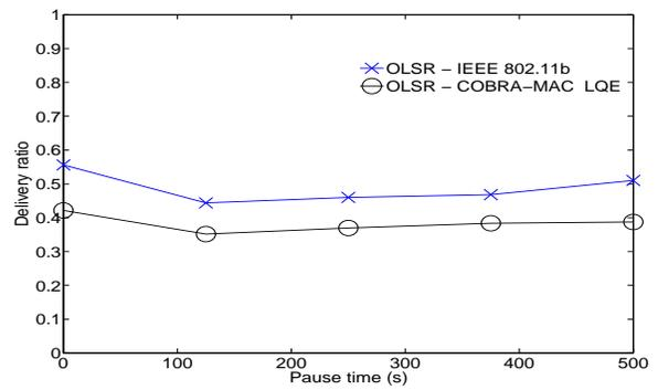
Fig. 101. Delivery ratio vs. Pause time, random waypoint mobility model, area is 320 m X 320 m, 30 nodes, 20 sources.
