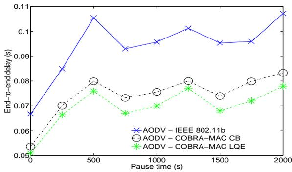
Fig. 34. End-to-end delay vs. Pause time, random waypoint mobility model, area is 320 m X 320 m, 20 nodes, 5 sources.
