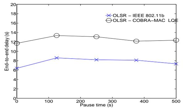
Fig. 102. End-to-end delay vs. Pause time, random waypoint mobility model, area is 320 m X 320 m, 30 nodes, 20 sources.
