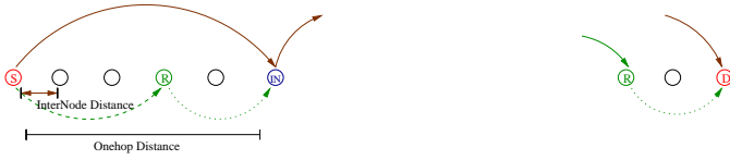
Fig. 7. Linear Topology showing the one hop and internode distances
