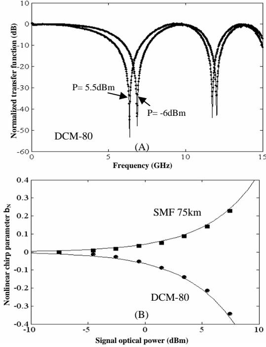
**Fig. 2, (A) Example of transfer function in a system with a dispersion compensating module (DCM-80) (B): Nonlinear chirp parameter  $b_N$  versus signal optical power for DCM-80 and 75km SMF. Dots: measured, continuous curves: calculated**
