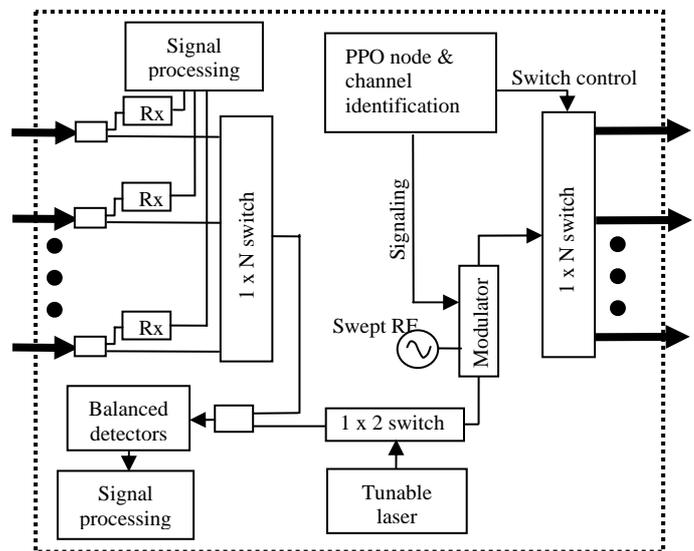
**Fig.1, PPO node using a tunable laser diode**
